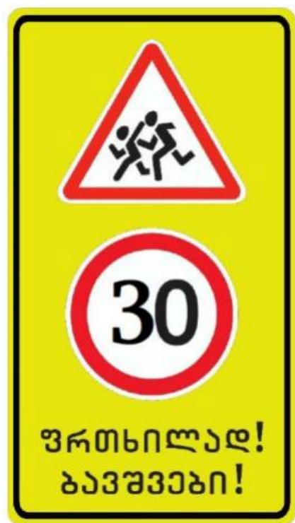
Sample of Coloured Road Signs Near Schools/Kindergartens – 30 kph
